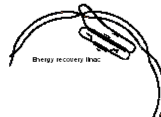
Schematic of electron-proton/ion collider based on the recirculating "linac-on-ring" concept.
